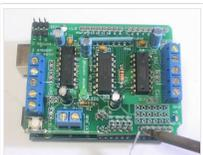
Solder in each pin of the header.
