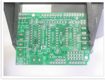
Place the motor shield PCB in a vise or other circuit-board holder and turn on your soldering iron to 700 degrees.
